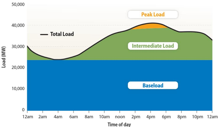
Fig. 6. Day electricity load curve in California, summer 2009 [19]
